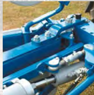
With the turnbuckle all side forces are balanced out for minimum draft requirement.
