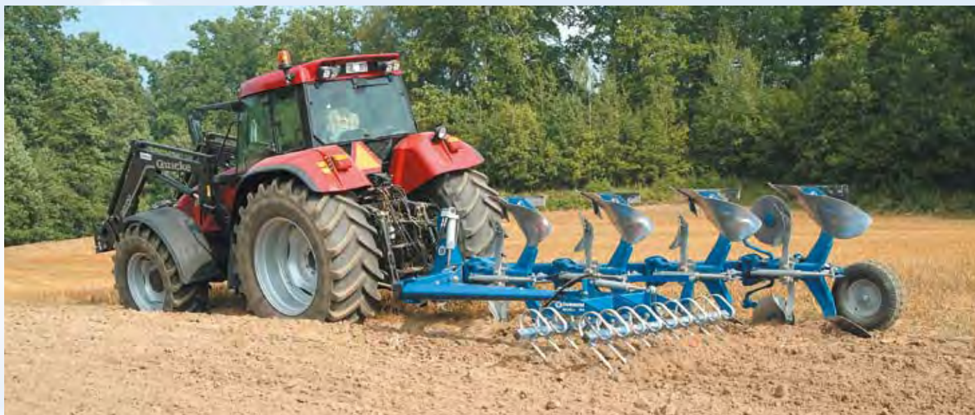
CX 490 H with Nivell furrow leveller. Ploughing and levelling in the same pass.
