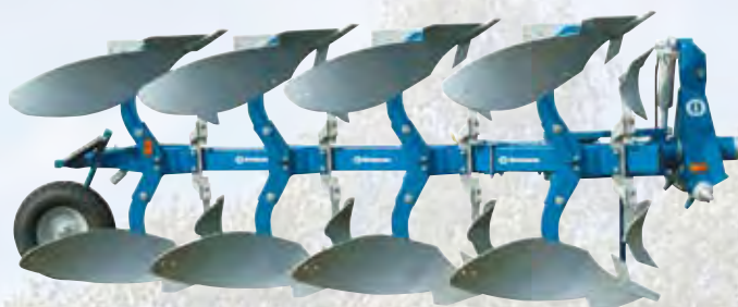
BX 490 F with EM-skimmers. Each leg and body is protected by a shear bolt.
