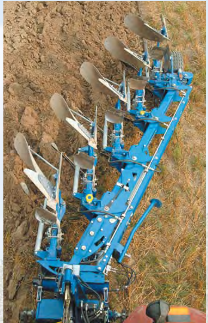
The centre of gravity is close to the tractor. Reducing the lift requirement.
