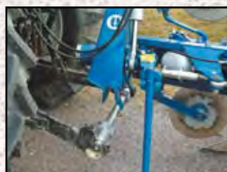
Quick coupling cross shaft for easy and safe connection.
