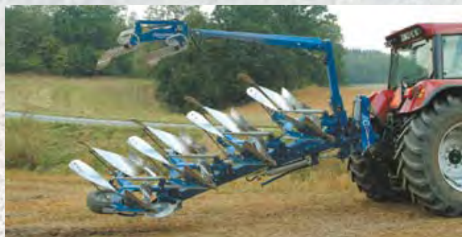
Bodies turning over the frame require slightly higher lift capacity. When the bodies are turning under the frame (see page 3) a lower lifting height is sufficient.
