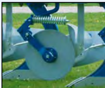
Spring loaded disc coulters. 18" or 20" plain or 20" rippled disc.
