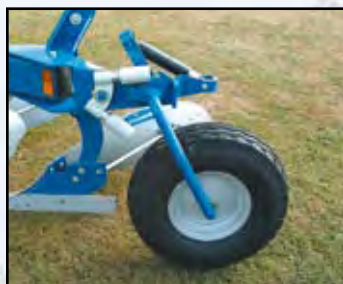
Depth wheel rubber 7.00 x 12. Diameter 645 mm, width 182 mm.
