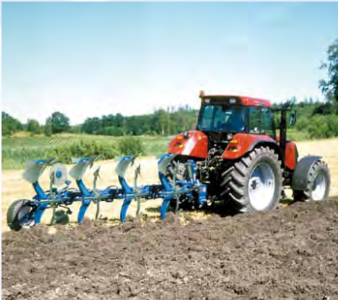
Vari Flex 490 H with high beams has extra clearance for heavy trash.
