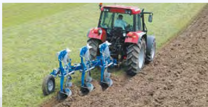
CX 390 H. XL-bodies and EG-skimmers perform a well closed finish.
