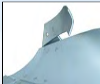
Trashboard. Good clearance for straw. Not recommended for sticky soils.
