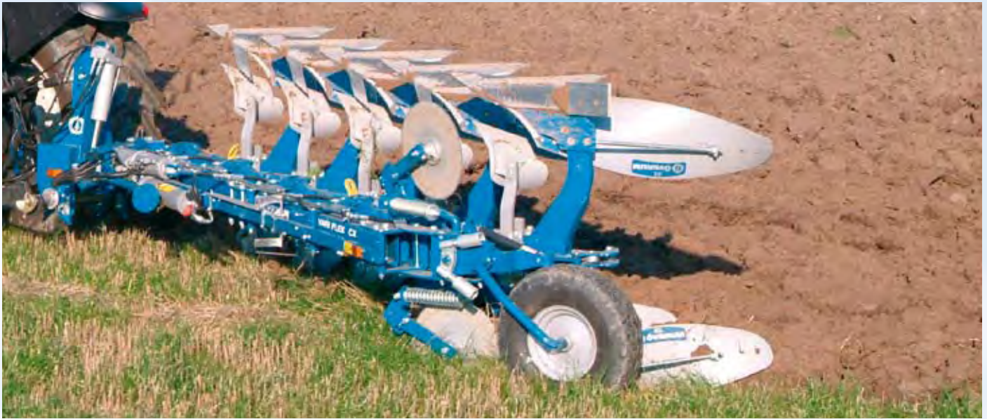
Vari Flex CX 580 H. Hydraulic furrow width adjustment from 1,5 to 2,25 m.
