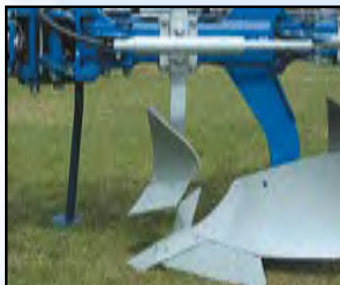
Skimmer EM. Handles large amounts of crop residues. Works best with fin coulters.
