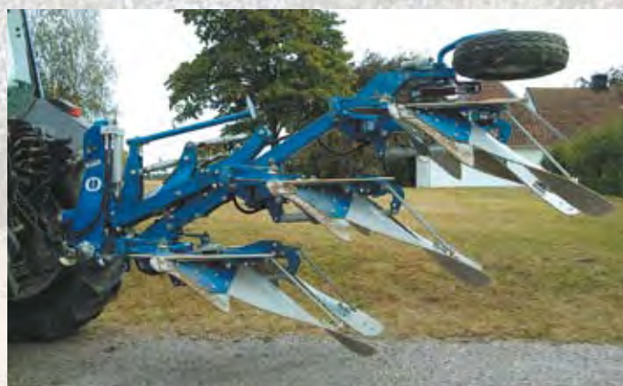
Due to the fact that the bodies are turning under the frame, the centre of gravity comes close to the tractor, and the plough becomes easy to lift.
