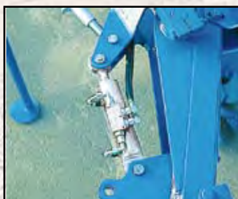
Hydraulic side adjustment BX. Front furrow width.
