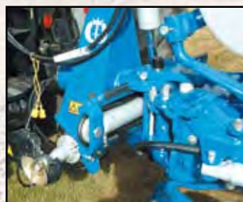
Hydraulic side adjustment CX/DX. Front furrow width.
