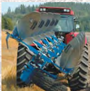
The automatic alignment secures a problem free turn over independent of furrow width setting.
