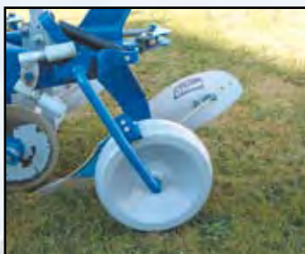
Depth wheel steel. Diameter 500 mm, width 160 mm.
