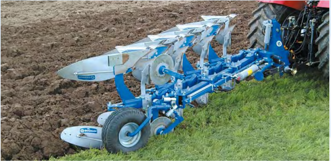
Vari Flex CX 490 H with hydraulic furrow width adjustment from 12 to 20 inches.
