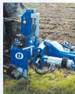
Heavy duty headstock with quick coupled cross shaft and alignment cylinder.
