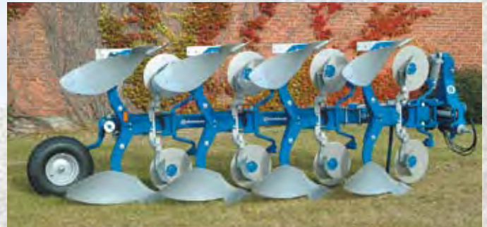
Vari Flex CX 490 F with fixed disc coulters and EG skimmers. Bodies as well as skimmers have individual shear bolts.
