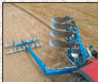
Nivell integrated furrow leveller from three to four furrows.
