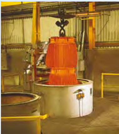
Carburizing of mouldboard blanks.
