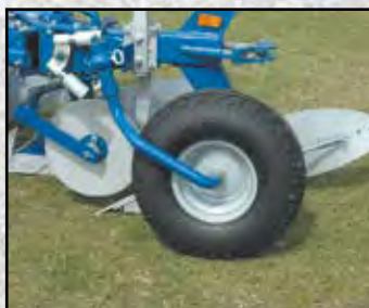
Combi wheel for depth control/transport 10.00 x 12. Diameter 710 mm, width 264 mm.
