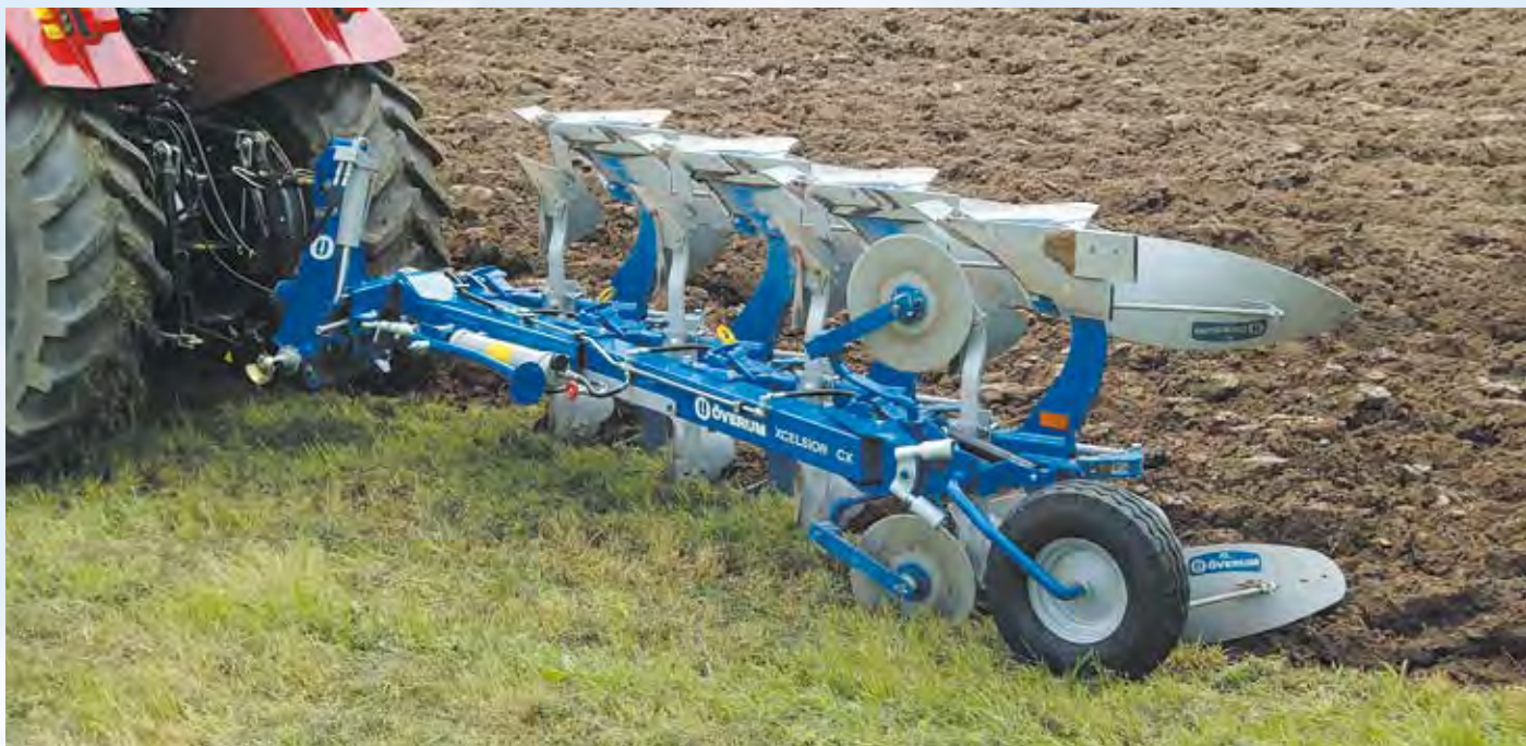
CX 490 H with EM-skimmers. 90 cm point to point clearance makes room for effective skimming equipment.
