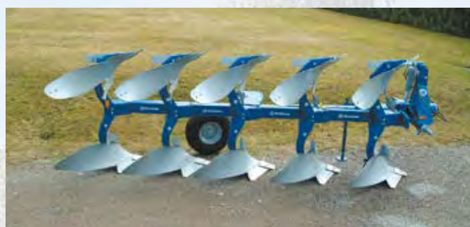
CX 590 F with trashboards and Combi wheel in forward position.
