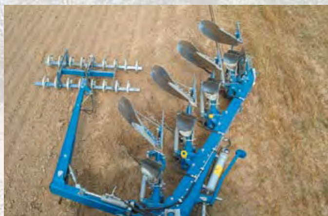
The frame profile becomes wider in the front as the forces are accumulated. The furrow width is adjustable in three steps.
