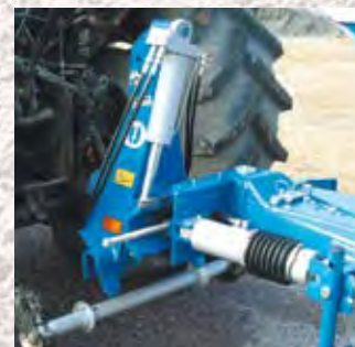
Quick coupling cross shaft for easy and safe connection.
