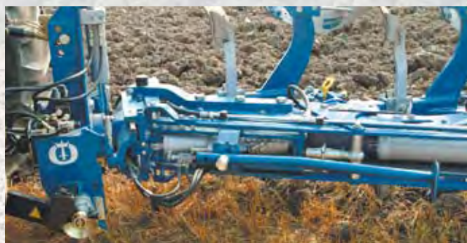
The double cylinder memorises the furrow width setting during the alignment and turnover action. The line of draft can be fine tuned in order to balance out all side forces and the plough pulls easy.
