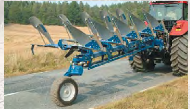
The new combi wheel is easy to set in transport position. Pressure is taken off the tractor for safe and rapid transport on rough roads.
