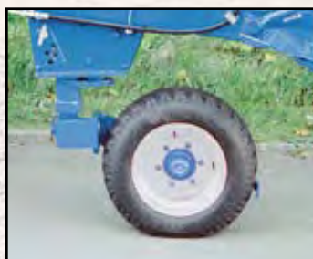
Combi wheel in forward position for Xcelisior DX models. Diameter 755 mm, width 275 mm.
