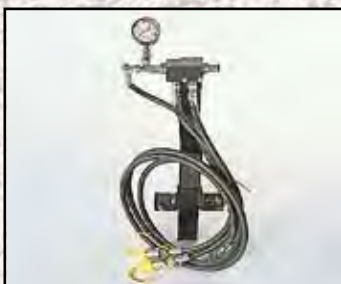
Stone release pressure adjustment set for on the go adjustment.
