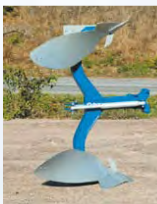
With high clearance profile beams large amounts of crop residues will flow through.
