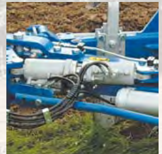
The double cylinder memorises the furrow width setting during the alignment and turnover action.
