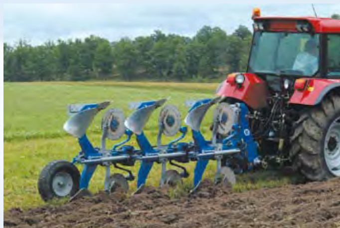
BX 380 H with XL-bodies, spring loaded disc coulters and EG-skimmers.
