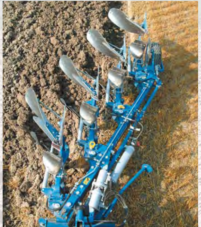
Precision drilling for the extensive bolt assembly has made it possible to use a heat-treated steel main frame tube.
